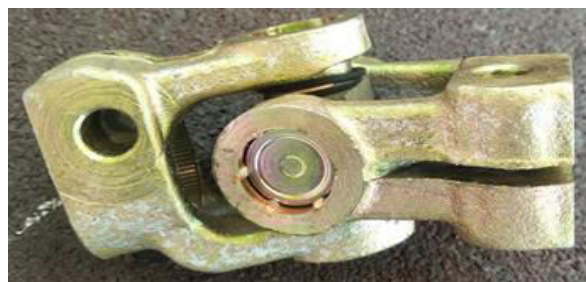
Fig.1 Universal Joint of Tata Sumo
