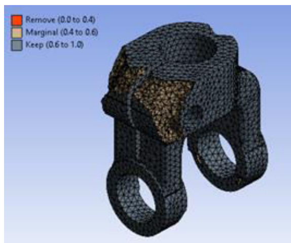
Fig.7 Material to be removed
