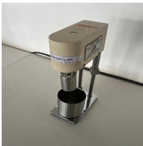
**Fig 3:** Hand crank viscometer
