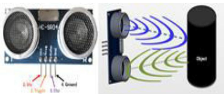
Fig.6: Ultrasonic Sensor
