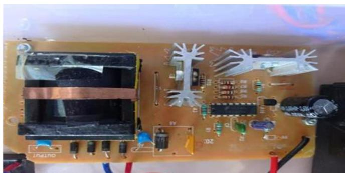
**Figure. 3: INVERTER CIRCUIT**
