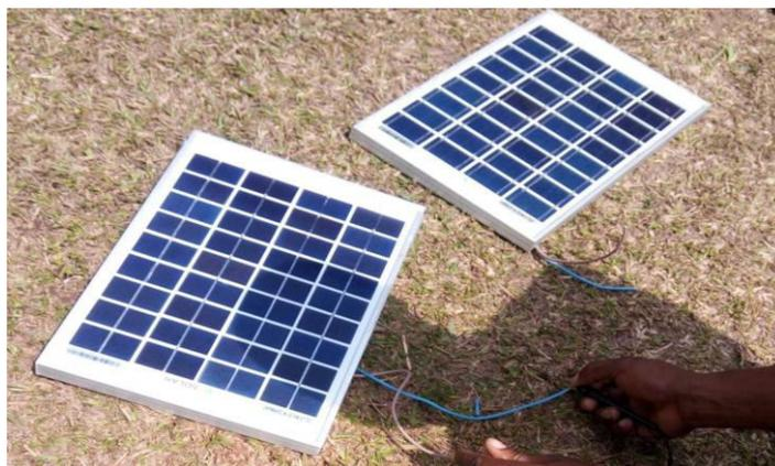
A solar cell panel, solar electric panel, photo-voltaic (PV) module or solar panel is an assembly of photo-voltaic cells mounted in a framework for installation.
