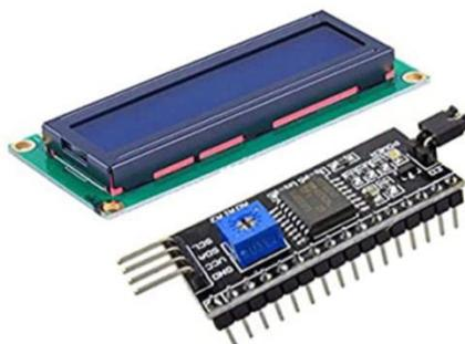
Fig.6: LCD with I2C
