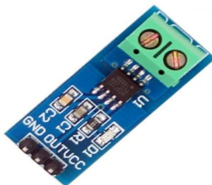
We've established a general idea of what current sensors are applicable for earlier. Well, with the ACS712 IC being able to detect both AC/DC current, it can be used in a wider range of applications apart from electrical appliances. Be it Arduino/other microcontroller usages, or industrial, commercial, and communication applications, it can be found applicable.
