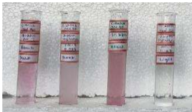
Photo 6: Effect of sunlight irradiation with respect to Dark condition and UV condition on photocatalytic degradation of Coralene Dark Red 2B in 300 minutes
