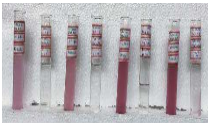
Photo 5: Effect of initial dye concentration on the photocatalytic degradation of Coralene Dark Red 2B MgZnAl 2 O 5 g/30ppm,40ppm,50ppm,60ppm
