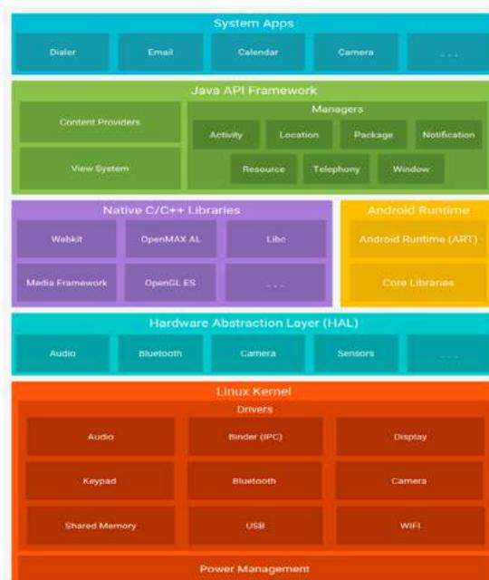
FIGURE 1. Android platform architecture [3]
