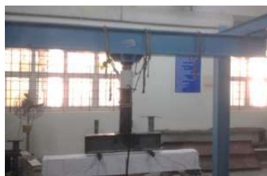
Fig. 3: Experimental test setup for beam testing
