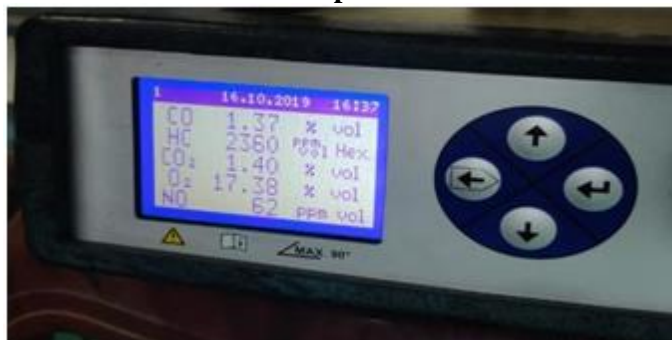
Fig 11 Five Gas test for modified two wheeler
