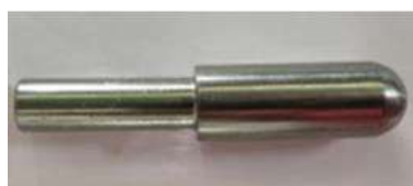
Fig. 2 Hemispherical form tool of diameter 15mm
