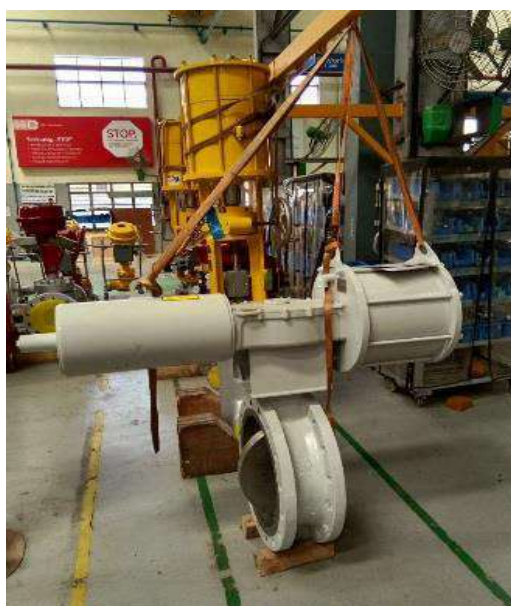
Fig. 1 Image of the existing valve holding set up
