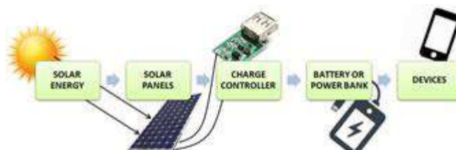
Fig. 3. Energy flow in the system
