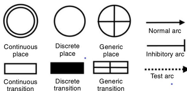
Fig. 6. Basic entities in the HFPNe architecture
