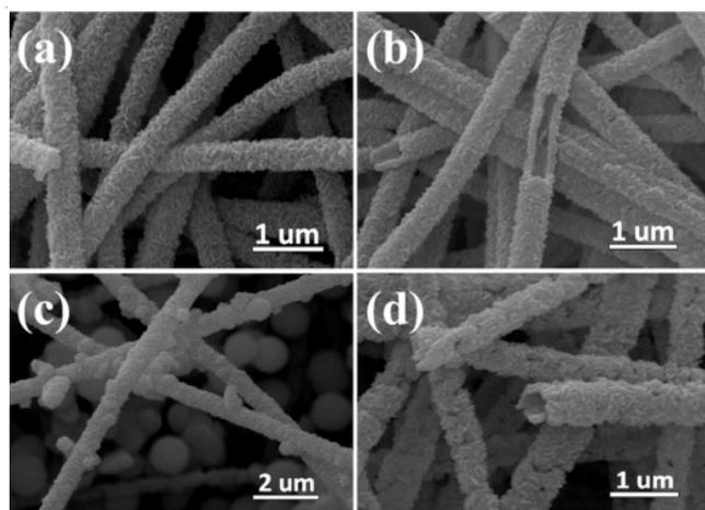
Fig. 1. SEM image of PANI/ $\text{V}_2\text{O}_5$  nanocomposite
