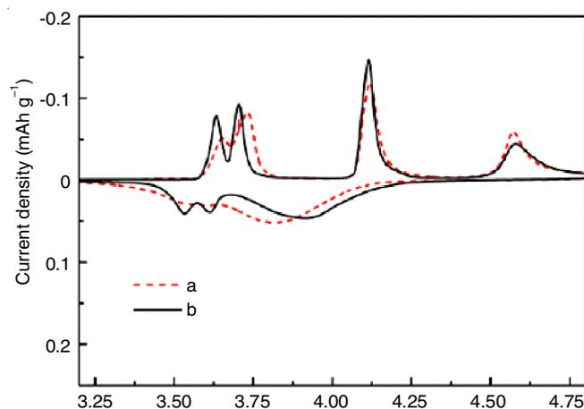
Fig. 3. Cyclic voltammogram curve of  $PANI/V_2O_5$  nanocomposite
