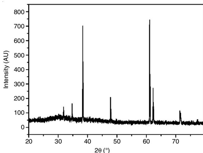
Fig. 2. XRD peaks of  $V_2O_5$ -PANI nanocomposite
