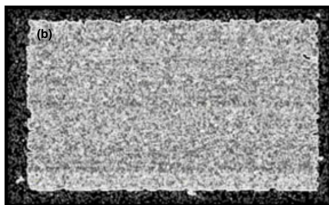
Fig. 10. Microscopic images of arecanut particle distribution (a) original microscopic image of particles (b) section view of particle distribution of arecanut shell
