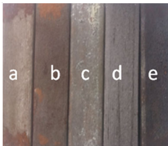
Fig. 4. Pictures of mild steels after corrosion in (a) 0.5 M acetic acid (b) 0.5 M formic acid (c) 0.5 M oxalic acid (d) 0.5 M citric acid (e) water
