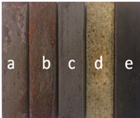
Fig. 5. Pictures of mild steel after corrosion in solutions containing (a) 10 % NaCl/90 % 0.5 M acetic acid (b) 10 % NaCl/90 % 0.5 M formic acid (c) 10 % NaCl/90 % 0.5 M citric acid (d) 10 % NaCl/90 % 0.5 M oxalic acid (e) 10 % NaCl/90 % water
