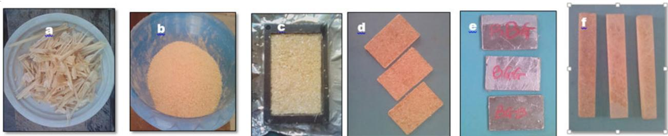
Plate 1: a - Raw Bagasse, b - grounded bagasse, c - Bagasse mat casting, d - Bagasse mats, e - bagasse/epoxy composite samples, f - DMA test specimens
