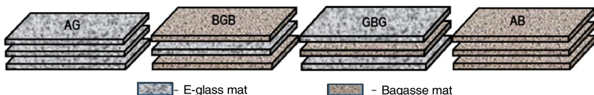
Fig. 1. Layering sequence model
