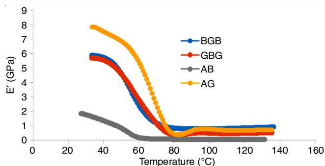
Fig. 2. Variation of storage modulus ( $E'$ ) as a function of temperature for AB, AG, BGB and GBG composites
