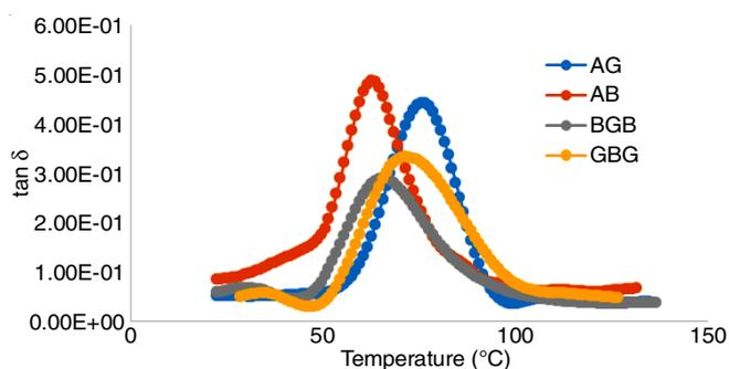
Fig. 4. Variation of damping factor ( $\tan \delta$ ) as a function of temperature for AB, AG, BGB and GBG composites
