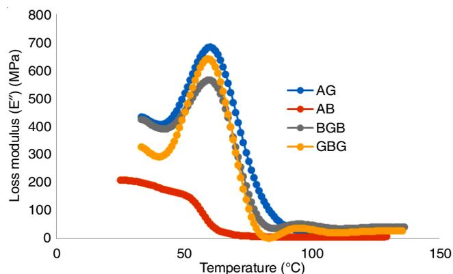
Fig. 3. Variation of loss modulus ( $E''$ ) as a function of temperature for AB, AG, BGB and GBG composites
