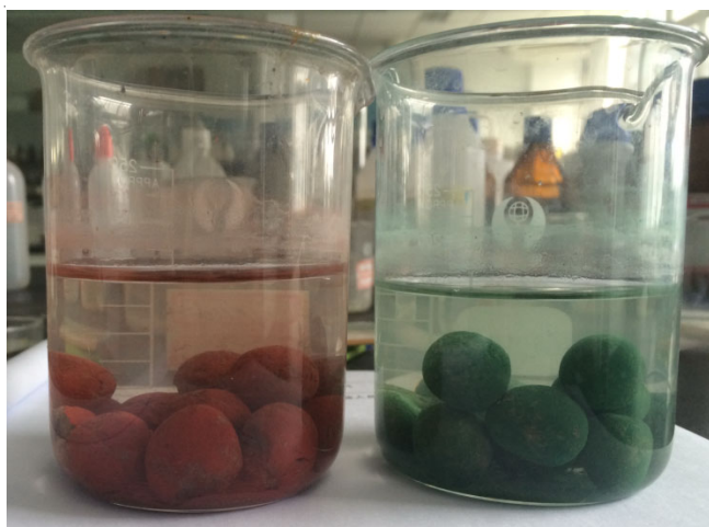
Fig. 2. Colour of the unburned and non-autoclaved ceramsite
