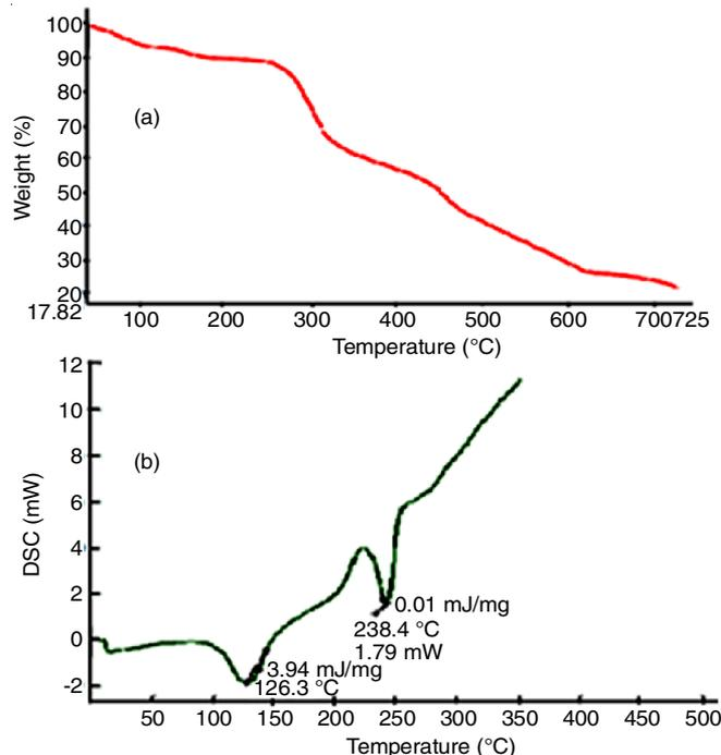
Fig. 3. (a) TGA/DTA and (b) DSC thermogram of the prepared chitosan
