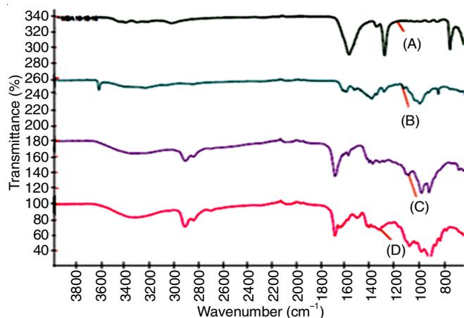
Fig. 2. FTIR spectrum of chitin (A), chitosan (B), G-1 (C), G-2 (D)
