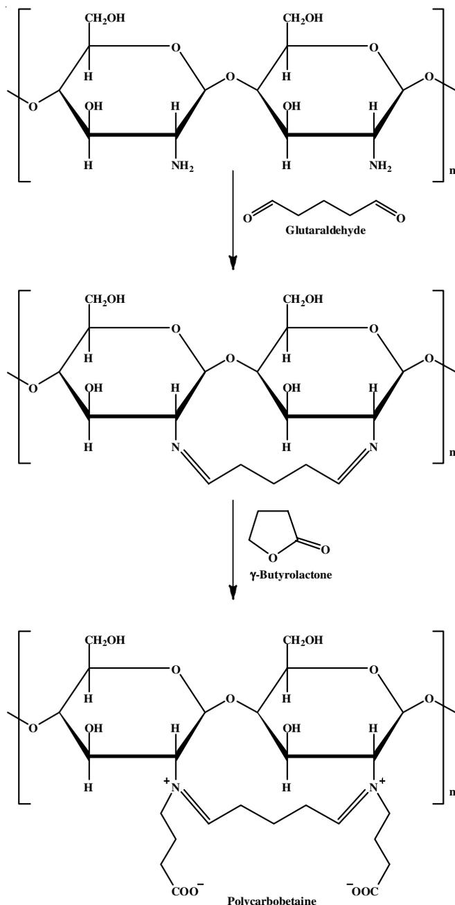
Fig. 1. Synthetic route for copolymer of chitosan and glutaraldehyde and its betainization to form polycarbobetaine
