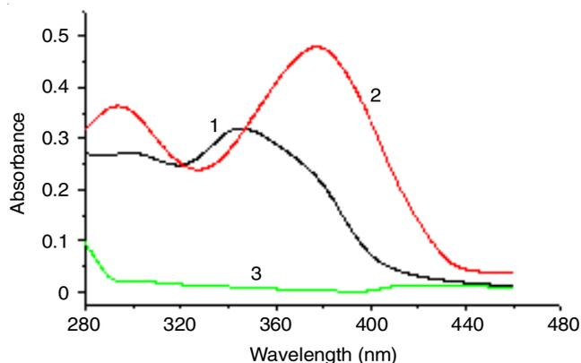
Fig. 2. Absorption spectra of doxycycline (1); Fe(III)-doxycycline (2); Reagent blank (3)
