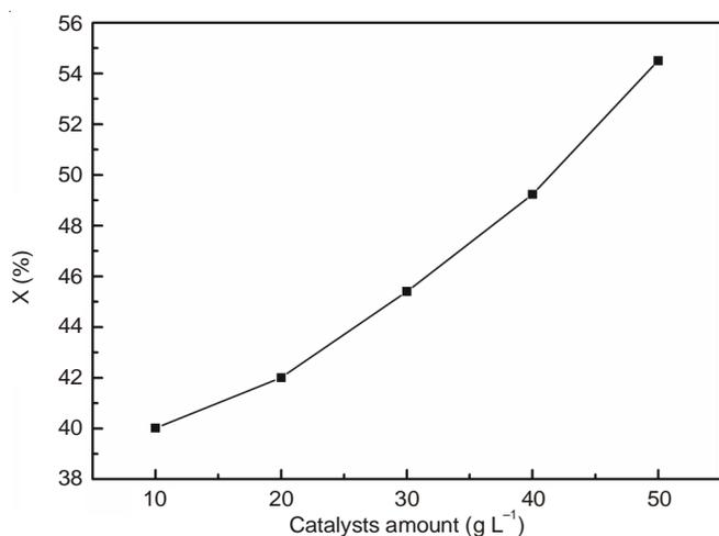
Fig. 4. Relation between catalyst amount and degradation rate of methyl orange under UV irradiation of 0.5 h
