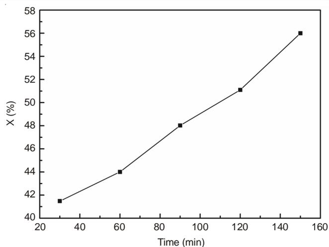
Fig. 5. Relationship between UV irradiation time and the degradation rate of methyl orange by catalysis
