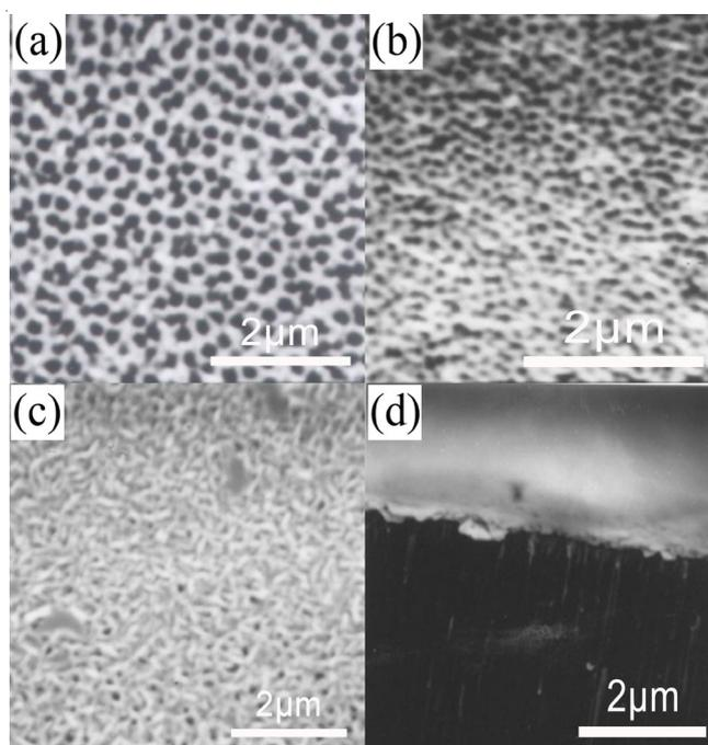
Fig. 2. SEM photograph of the surface of the template after different immersion time: (a) 0 min; (b) 6min; (c) 8 min; (d) side view of (b)
