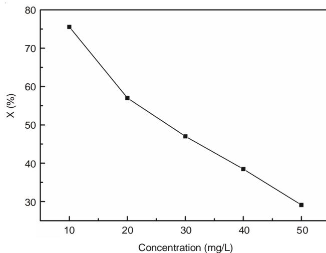
Fig. 6. Relation between different concentrations of catalyst and the degradation rate of methyl orange under UV irradiation of 0.5 h
