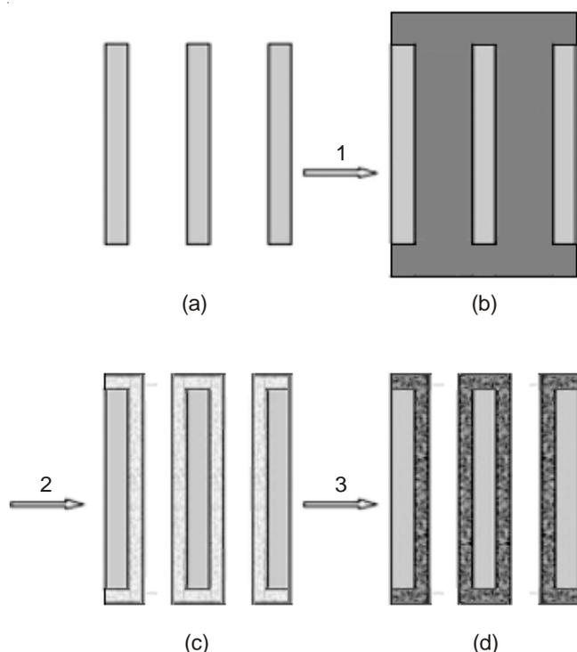
Fig. 1. Preparation of ZnO nano-tube; (a) the porous anodic alumina template; (b) the porous anodic alumina template immerse in a ZnO sol; (c) the ZnO absorbed on the wall of anodic alumina template after drying; (d) after high-temperature calcined there was formed a nano-porous ZnO thin films with nanotube structure (*i.e.* the catalyst) inside the nanopores of the anodic aluminum template
