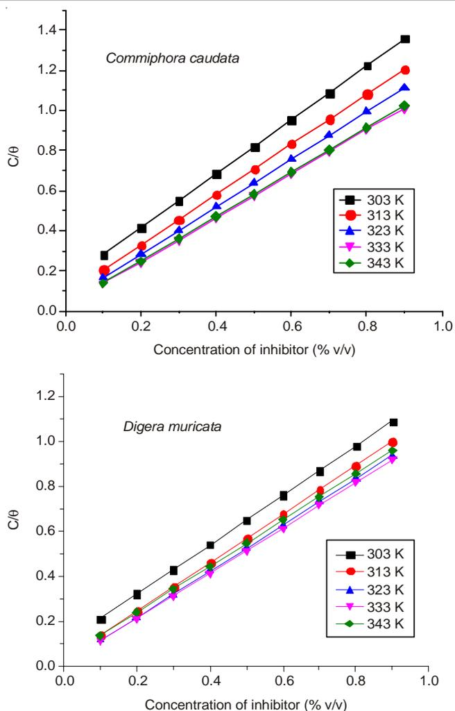
Fig. 3. Langmuir adsorption isotherm plot for the different concentrations of *Commiphora caudata* and *Digera muricata* extract on the mild steel in 1 M HCl at 303 and 333 K
