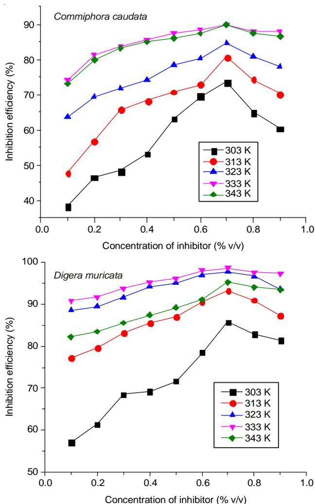
Fig. 1. Variation of inhibition efficiency of *Commiphora caudata* and *Digera muricata* extract, at different concentrations, on mild steel in 1 M HCl at different temperatures
