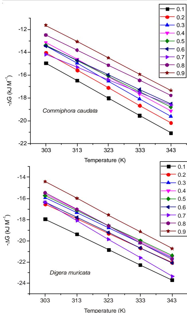
Fig. 2.  $\Delta G_{ads}$  as a function of temperature in the presence of *Commiphora caudata* and *Digera muricata* extract in 1 M HCl
