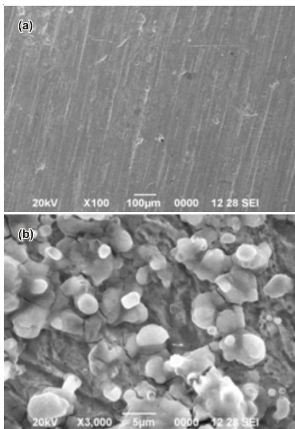
Fig. 4. SEM photograph of (a) polished mild steel and (b) mild steel immersed in 1 M HCl
