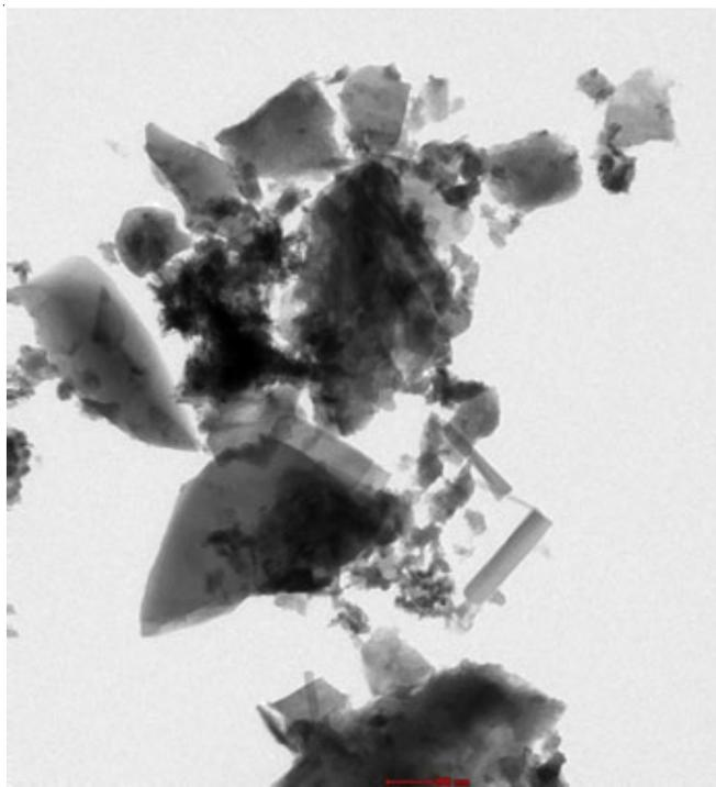
Fig. 2. TEM analysis of ZnO nanoparticles of leaf extract of *R. cordifolia*
