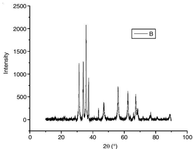
Fig. 1. X-ray diffraction pattern of ZnO nanoparticles of leaf extract of *R. cordifolia*
