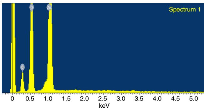
Fig. 3. EDX pattern of synthesized ZnO nanoparticles of leaf extract of *R. cordifolia*
