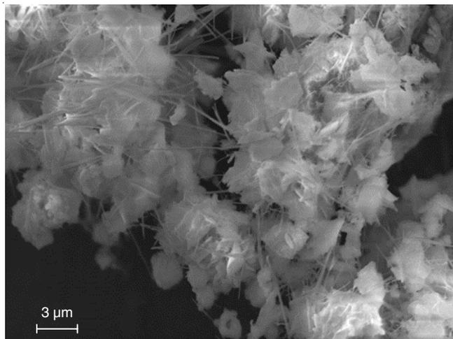
Fig. 4. SEM analysis of ZnO nanoparticles of leaf extract of *R. cordifolia*
