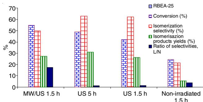
Fig. 8. Comparison of activities of different combined systems with microporous zeolite RBEA-25 in the conversion of geraniol. Reaction conditions: catalyst loading – 0.92 mol of geraniol/g catalyst, argon atmosphere, run time – 1.5 h, 5.0 h, temperature – 80 °C, US (350 W), US/MW (300 W/550 W)
