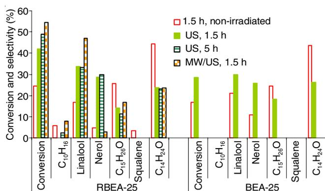
Fig. 5. Comparison of catalytic activities (at 80 °C, medium – Ar) of non-irradiated and irradiated with ultrasound zeolites (RBEA-25 and BEA-25) in reaction of geraniol conversion by • irradiation during 1.5 h, US power- 350 W, • irradiation during 5 h, • with combined US/MW irradiation during 1.5 h, US power - 300 W, MW power-550 W
