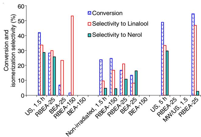
Fig. 7. Geraniol conversion under US (350 W) and combined US/MW (300 W/550 W) irradiations in the presence of micro- and micro-mesoporous beta-type zeolites. Effect of ultrasound irradiation time on degree of geraniol conversion and selectivity to linalool and to nerol; reaction conditions – catalyst loading – 0.92 mol of geraniol/g catalyst, argon atmosphere, run time 1.5 h, 5.0 h, temperature 80 °C
