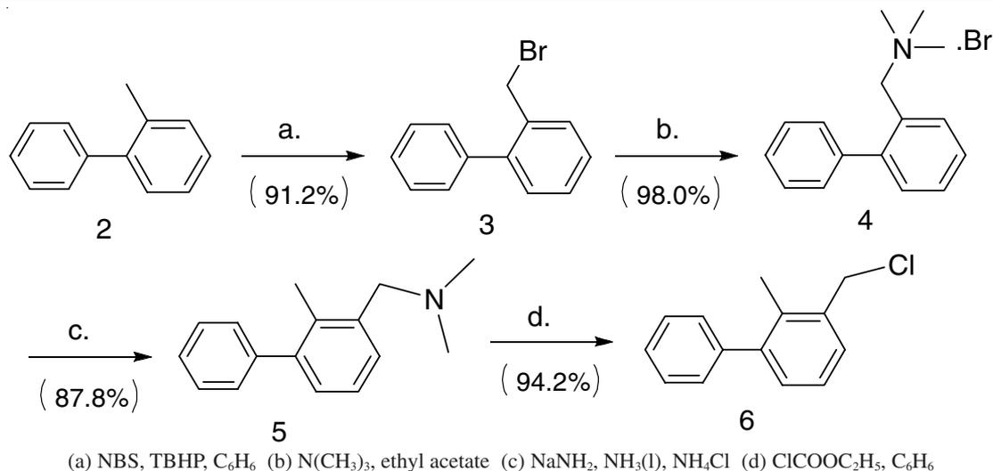
**Scheme-II:** Synthetic scheme of 3-(chloromethyl)-2-methyl-1,1'-biphenyl from 2-methyl-1,1'-biphenyl
