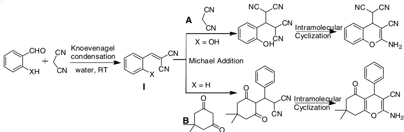
Scheme-II: Proposed mechanism of current cascade protocol
