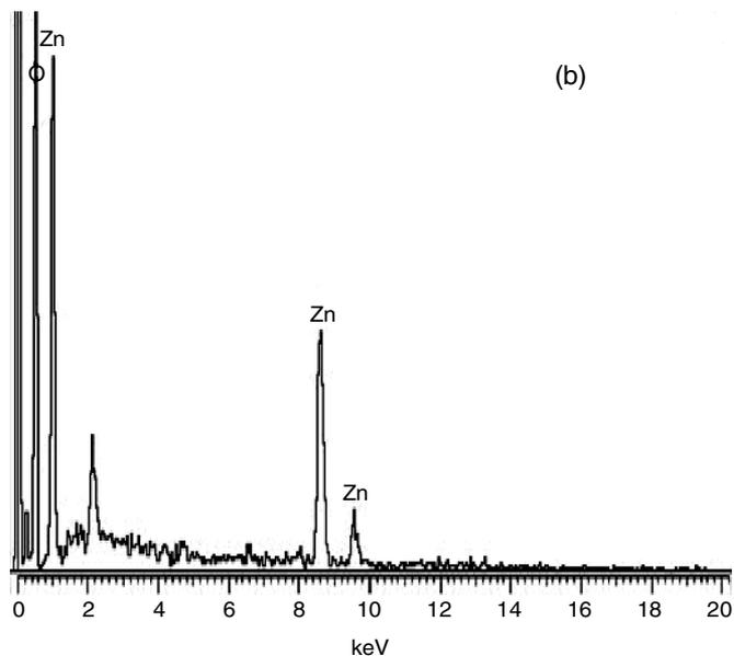
Fig. 3. SEM image (a) and EDX (b) of bio derived ZnO nanoparticles
