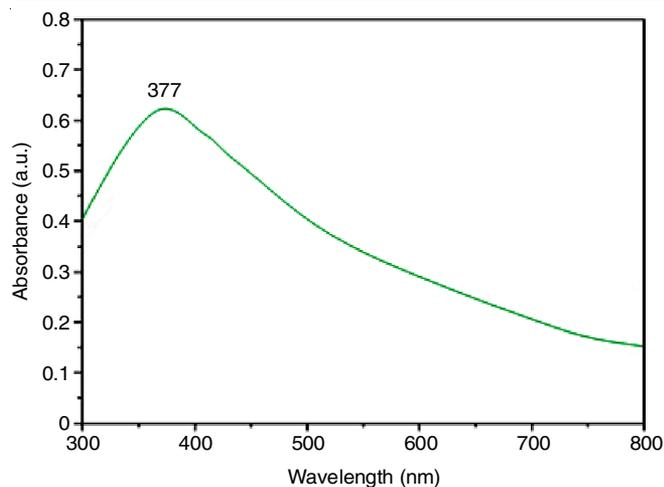
Fig. 1. UV-visible absorption spectrum of ZnO nanoparticles
