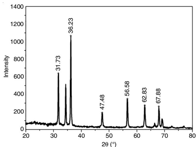
Fig. 2. XRD pattern of bio derived ZnO nanoparticles
