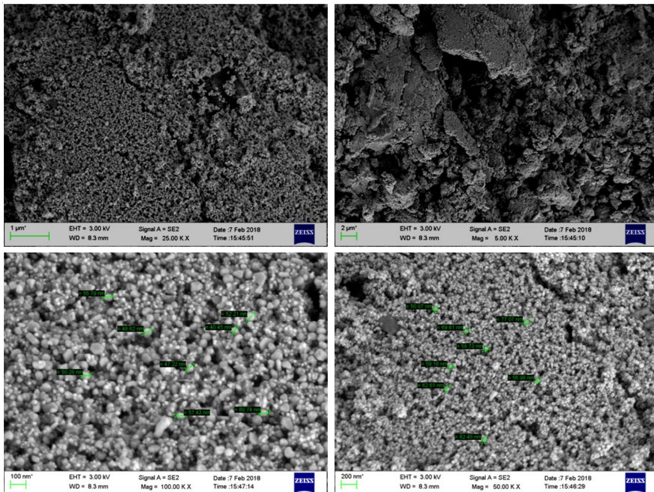
Fig. 3. Scanning electron microscopy images of AgNPs synthesized using *Coldenia procumbens* Linn. extract
