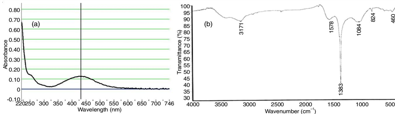
Fig. 1. (a) UV-Visible spectrum of AgNPs, (b) FTIR spectrum of AgNPs
