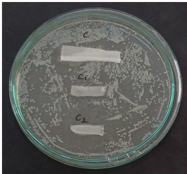
Fig. 6. Antimicrobial activity of untreated cotton (C) and ZnO-treated samples (C1 and C2)
