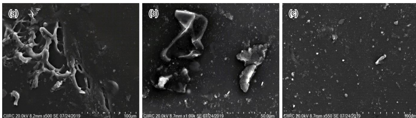
Fig. 9. SEM image of epoxy coated mild steel in acidic condition
