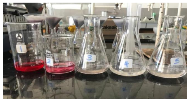
Fig. 4. Colour of solutions resulted after adsorption with a known amount of adsorbent 1. 0 g, 2. 0.02 g, 3. 0.08 g, 4. 0.1 g, and 5. 0.12 g
