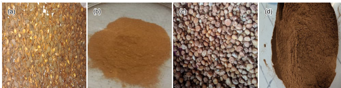
Fig. 1. Results of chopping water-free fruit flesh (a), seeds (b) and results of sieving powder with a size of 60 mesh for fruit flesh (c) and seeds (d)
