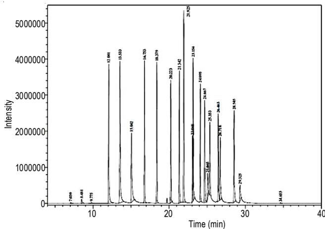
Fig. 1. GC-ECD chromatogram of standard
