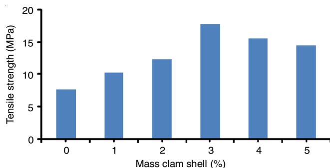
Fig. 1. Effect of variations in the composition of clam shells on the tensile strength properties of polyester composites
