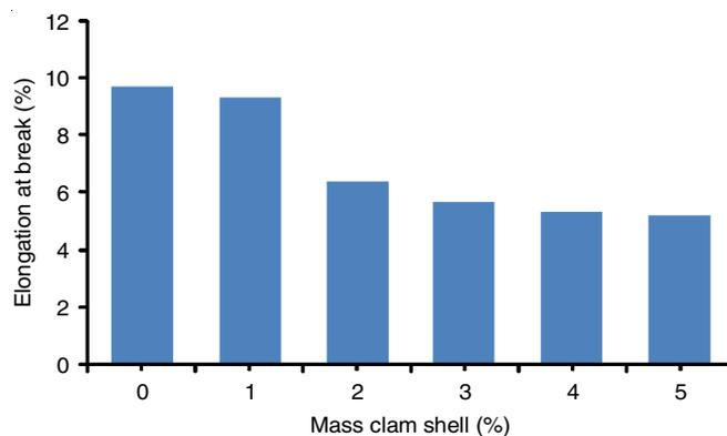
Fig. 2. Effect of clam shell filler composition variations on elongation at break properties polyester composites
