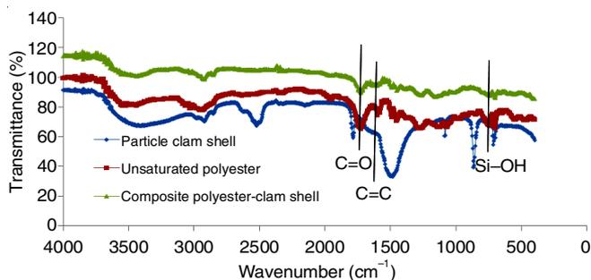
Fig. 4. Analysis of Fourier transform infrared polyester composites filled with clam shells, Unsaturated polyester and particle clam shell
