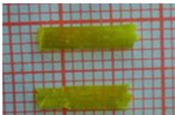
Fig. 1. As-grown crystal of 4-methylpyridinium picrate
