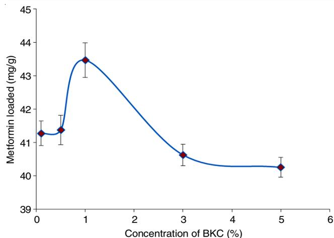
Fig. 3. Amount of metformin hydrochloride loaded on BKC modified clinoptilolite. Error bars show the standard deviation (n = 4)
