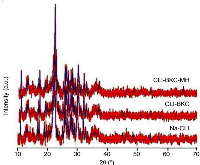
Fig. 2. XRD pattern of Na-clinoptilolite (Na-CLI), clinoptilolite-benzalkonium chloride (CLI-BKC) and clinoptilolite-benzalkonium chloride-metformin hydrochloride (CLI-BKC-MH)
