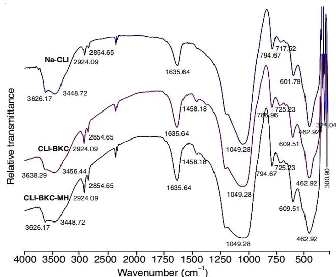
Fig. 1. FTIR spectra of Na-clinoptilolite (Na-CLI), clinoptilolite-benzalkonium chloride (CLI-BKC) and clinoptilolite-benzalkonium chloride-metformin hydrochloride (CLI-BKC-MH)
