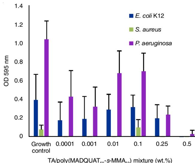
Fig. 6. Effect of tannic acid (0.1 wt%)/poly(MADQUAT<sub>50</sub>-s-MMA<sub>50</sub>) mixtures on biofilm developed under static condition for 18 h. The results are expressed as the mean of 24 replicate wells involving three biological replicates for each strain. Error bars indicate the standard error of the mean
