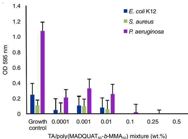
Fig. 8. Effect of tannic acid (0.1 wt%)/poly(MADQUAT<sub>50-b-MMA<sub>50</sub></sub>) diblock polymer mixtures on the biofilm developed under static condition for 18 h. The results are expressed as the mean of 24 replicate wells involving three biological replicates for each strain. Error bars indicate the standard error of the mean
