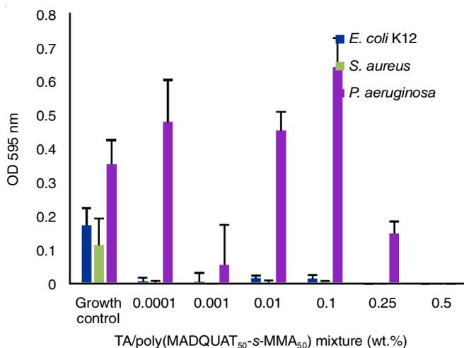
Fig. 7. Effect of tannic acid (0.1 wt%)/poly(MADQUAT<sub>50-s-MMA<sub>50</sub></sub>) mixtures on biofilm developed under static condition for 18 h. The results are expressed as the mean of 24 replicate wells involving three biological replicates for each strain. Error bars indicate the standard error of the mean
