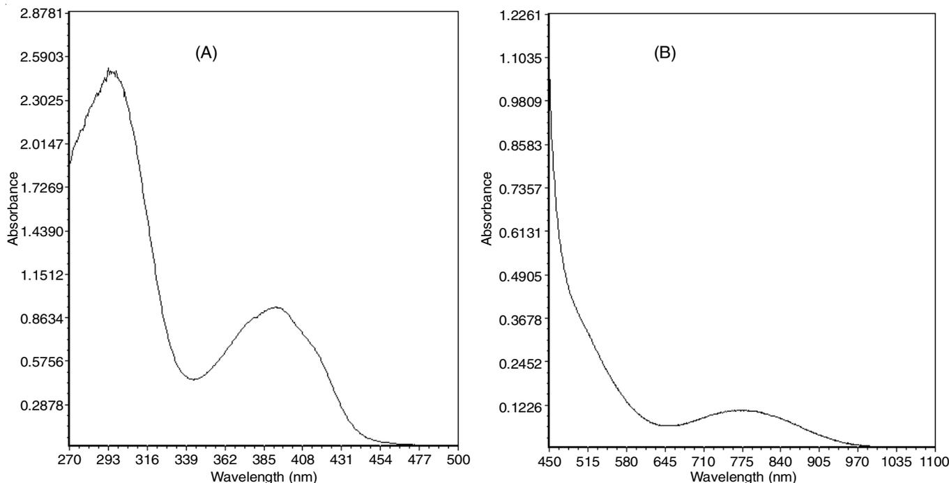
Fig. 1. UV-visible spectra of V(APBH)Cl<sub>3</sub> (A) in the UV region and (B) in the visible region. In total three peaks are observed in A and B
