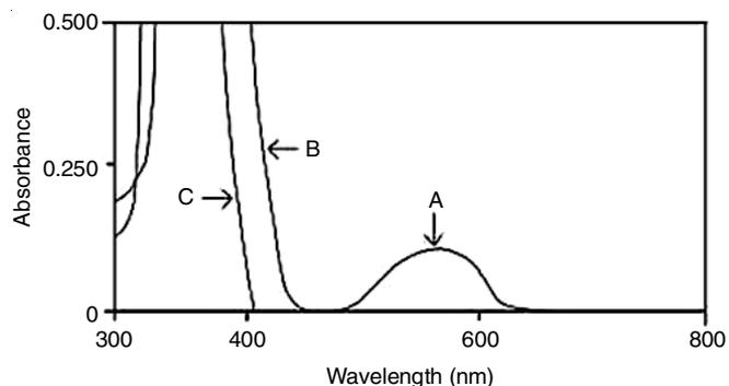
Fig. 4. Absorption spectra of (A)  $8 \mu\text{g mL}^{-1}$  of sodium cefotaxime versus reagent blank, (B)  $8 \mu\text{g mL}^{-1}$  of sodium cefotaxime versus distilled water, and (C) blank versus distilled water
