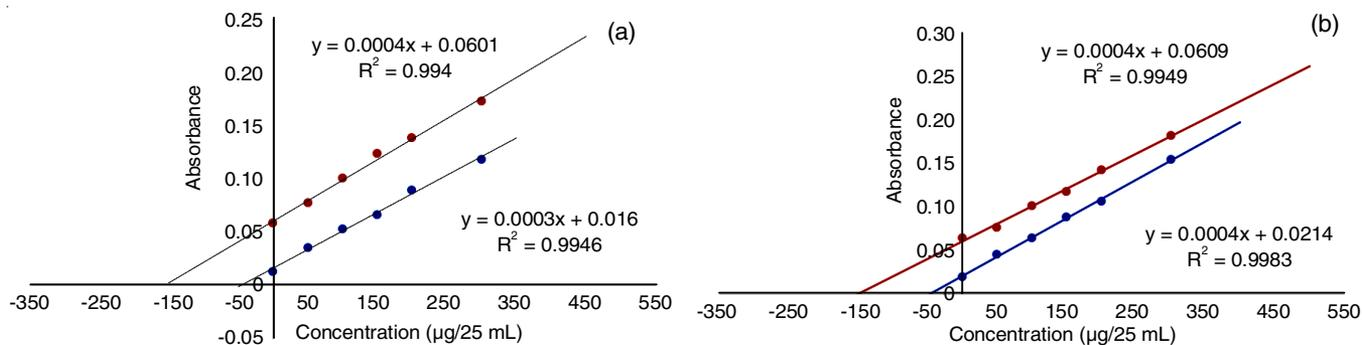
Fig. 9. Graphs of standard addition method for determination of sodium cefotaxime in (a) cefotaxime and (b) Belaksim injections
