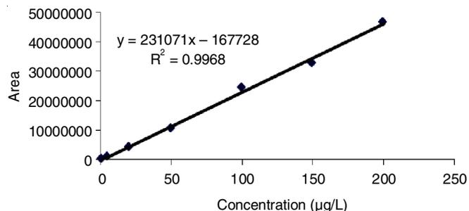
Fig. 3. Calibration graph of sodium cefotaxime by the HPLC method
