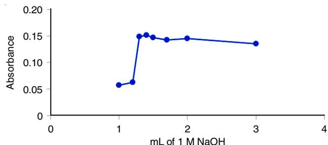
Fig. 6. Effect of NaOH amount on absorbance
