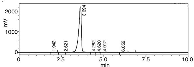
Fig. 12. Chromatogram of sodium cefotaxime using  $1 \text{ min mL}^{-1}$  as flow rate
