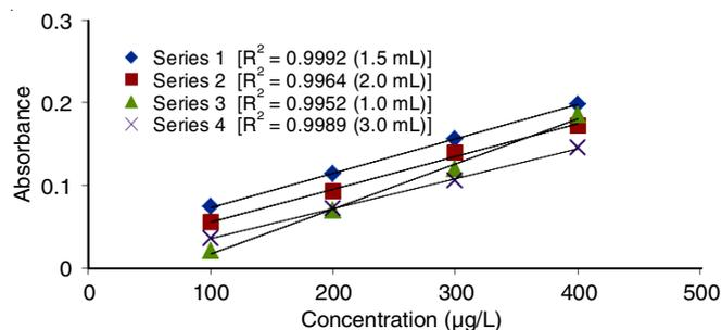
Fig. 5. Effects of 8-hydroxyquinoline amount on absorbance
