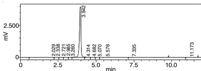
Fig. 11. Chromatogram of sodium cefotaxime using acetonitrile:phosphate buffer solution pH 5.2 (60:40) (v:v) as a mobile phase
