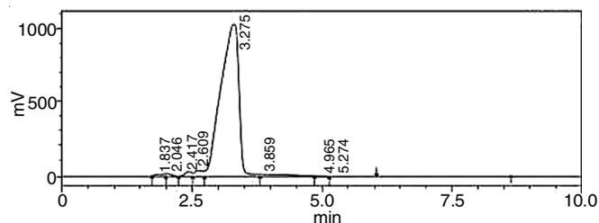
Fig. 13. Chromatogram of sodium cefotaxime using phosphate buffer solution at pH 3.5 with acetonitrile as mobile phase
