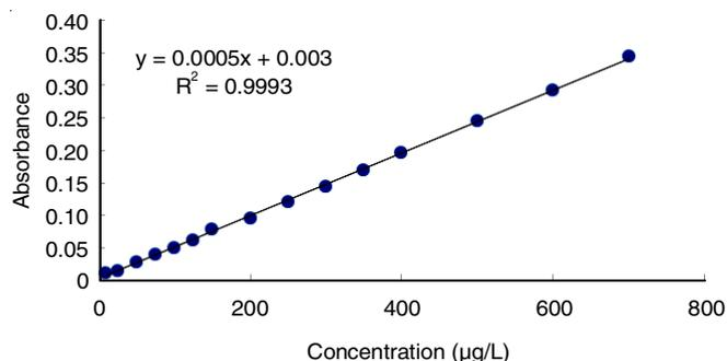
Fig. 2. Calibration curve for sodium cefotaxime determination
