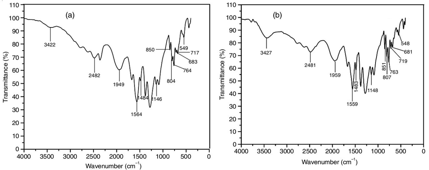
Fig. 3. FT-IR spectra of (a) pure KHP and (b) AAKHP crystals
