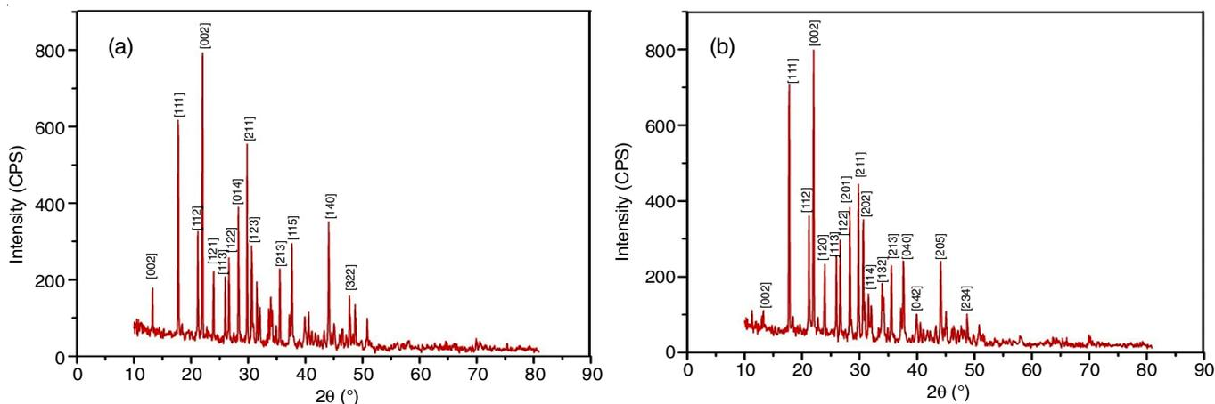
Fig. 2. Powder XRD patterns of (a) KHP crystal and (b) AAKHP crystal
