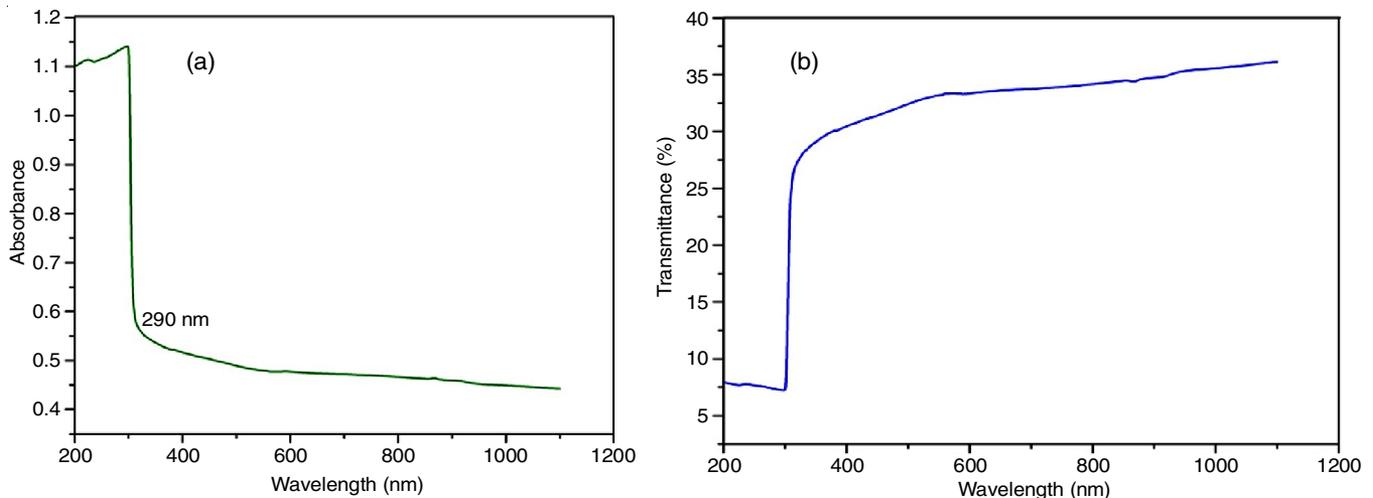
Fig. 4. Optical absorption (a) and optical transmittance (b) spectra of AAKHP crystal
