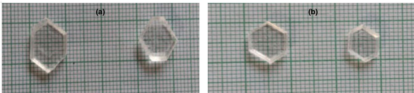
Fig. 1. As grown crystal of (a) pure KHP and (b) AAKHP crystals
