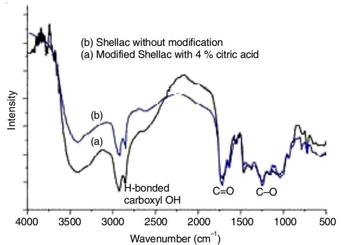
Fig. 2. FTIR spectra of non-modified Shellac and modified Shellac citric acid of 4 %
