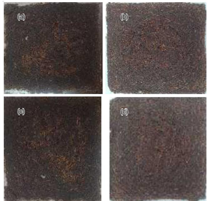
Fig. 3. (a) Non-modified Sh-Bg biocomposite, (b) Sh-Bg biocomposite modified with citric acid with a ratio of 60:40 %, (c) Sh-Bg biocomposite modified with citric acid with a ratio of 40:60 %, (d) Sh-Bg modified with citric acid with a ratio of 50:50 %
