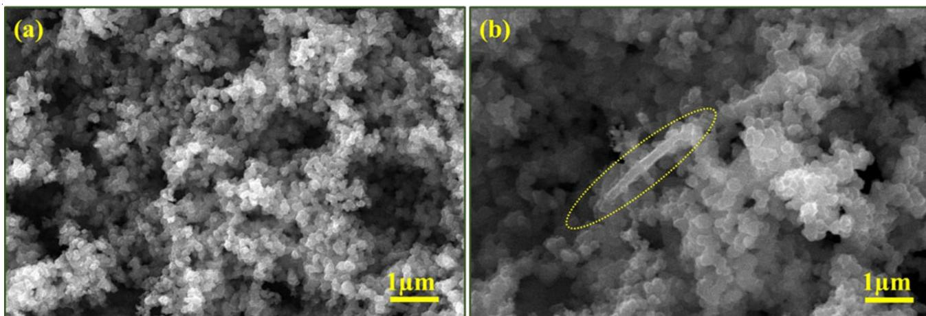
Fig. 3. SEM micrographs of (a) PPy and (b) PPy/ZnO/SWCNT nanocomposite
