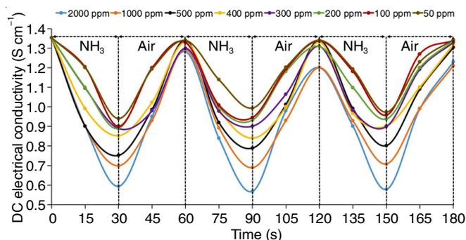
Fig. 8. Reversibility of the sensor on alternate exposure of ammonia and air at different concentrations
