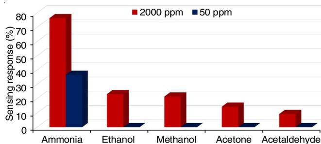
Fig. 9. Selectivity of the sensor at 2000 ppm and 50 ppm of ammonia
