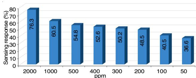
Fig. 7. Sensing response of the sensor towards ammonia at different concentrations
