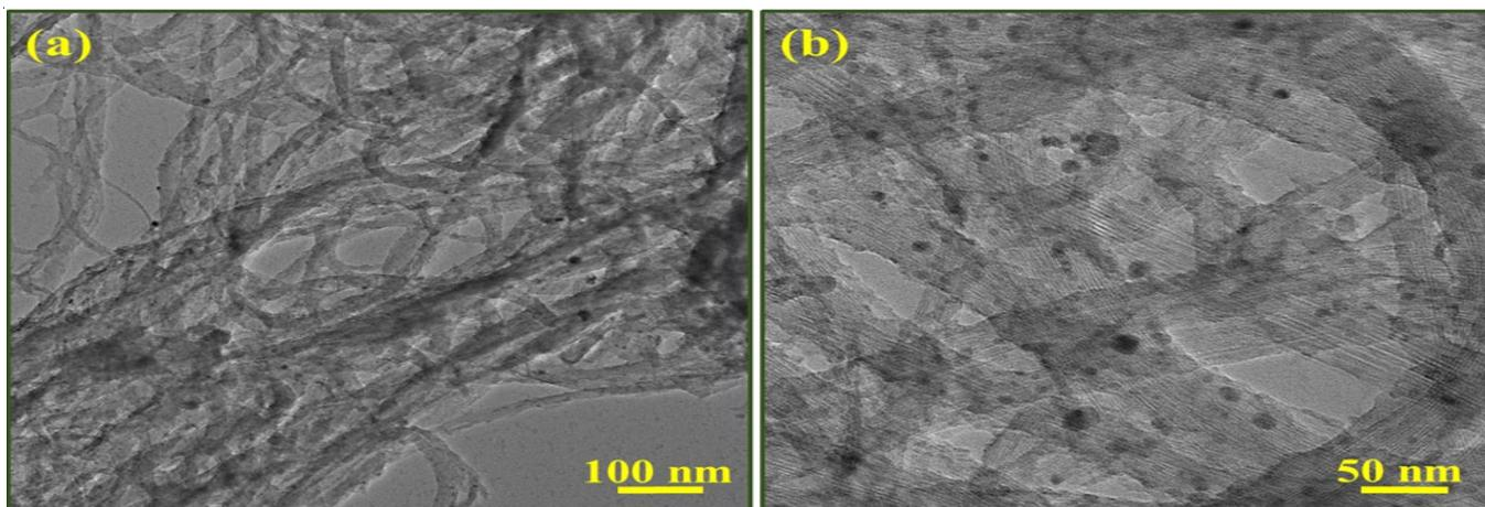
Fig. 4. TEM micrographs PPy/ZnO/SWCNT nanocomposite at different magnifications
