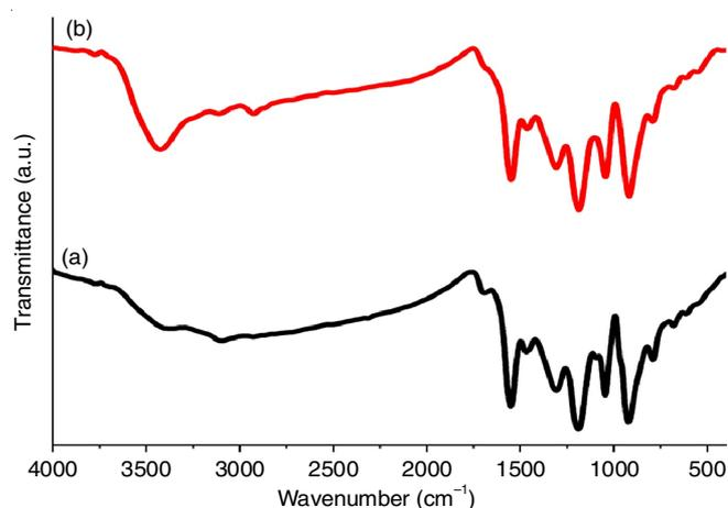
Fig. 1. FT-IR spectra of (a) PPy and (b) PPy/ZnO/SWCNT nanocomposite
