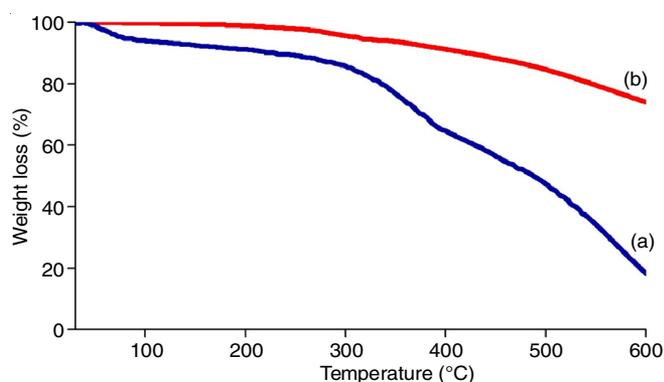
Fig. 5. Thermograms of (a) PPy and (b) PPy/ZnO/SWCNT nanocomposite
