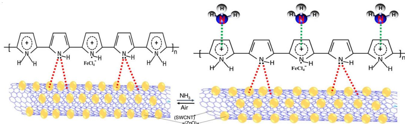
Fig. 11. Proposed sensing mechanism concerning the electronic interaction of charge carriers of PPy with lone pairs of ammonia molecules
