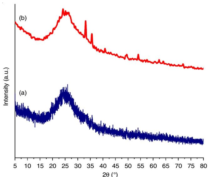
Fig. 2. XRD spectra of (a) PPy and (b) PPy/ZnO/SWCNT nanocomposite
