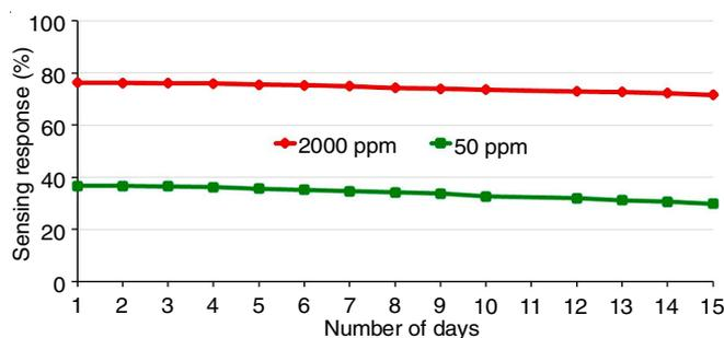
Fig. 10. Stability of the sensor at 2000 ppm and 50 ppm of ammonia
