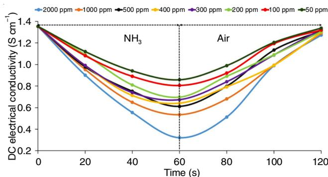
Fig. 6. Variation in DC electrical conductivity of sensor on alternate exposure of ammonia and air at different concentrations
