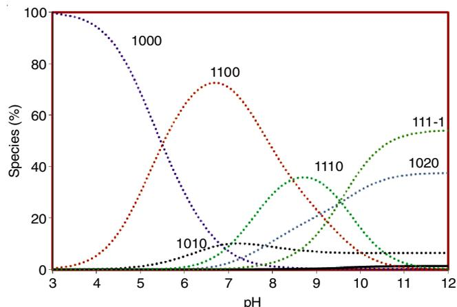
Fig. 2. Concentration distribution of various species as a function of pH in Cu(II)-piroxicam-Serine complexes
