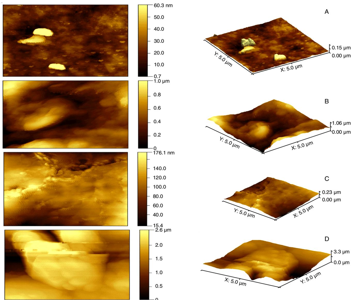
Fig. 5. AFM images of the membrane pure PVA, binary PVA/PEG and blend membrane PVA/PEG/KC1 (10%), PVA/PEG/KC2 (20%)
