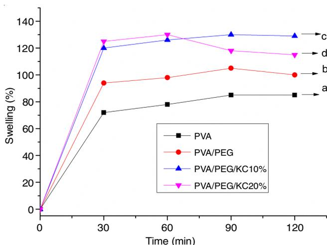
Fig. 6. Swelling behaviour of the membrane pure PVA, binary PVA/PEG and blend membrane PVA/PEG/KC1 (10%), PVA/PEG/KC2 (20%)
