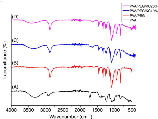
Fig. 2. FTIR spectra of (A) Pure PVA (B) PVA/PEG and blend (C) PVA/PEG/KC1, (D) PVA/PEG/KC2
