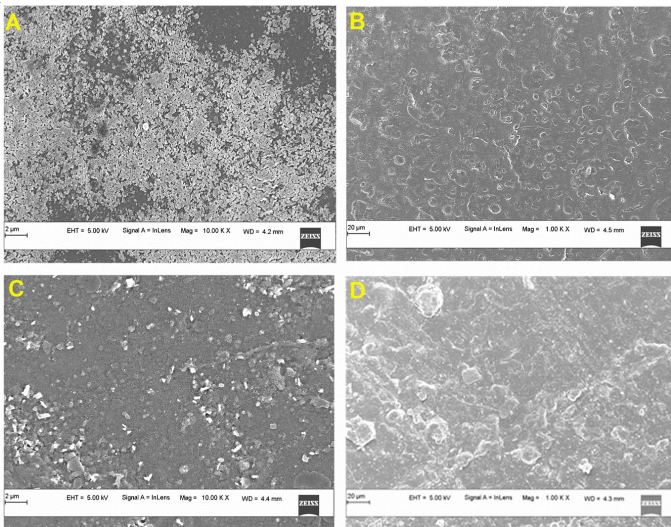
Fig. 1. FESEM images of film pure (A) PVA binary (B) PVA/PEG and blend (C) & (D) PVA/PEG/KC1 & 2, respectively in the range scale bar of 2-20  $\mu\text{m}$
