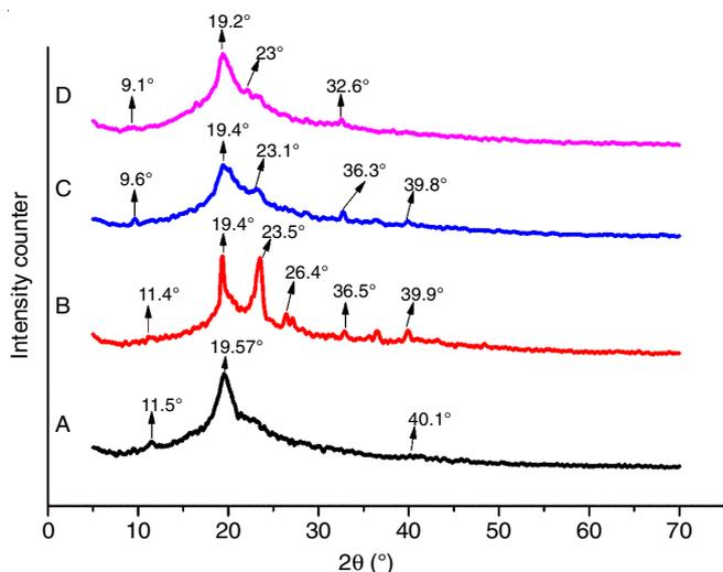
Fig. 4. XRD of membrane pure PVA binary PVA/PEG and blend membrane PVA/PEG/KC1 (10%), PVA/PEG/KC2 (20%)
