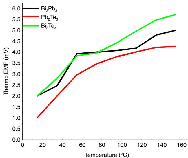
Fig. 1. Thermo-emf generation in normal mode
