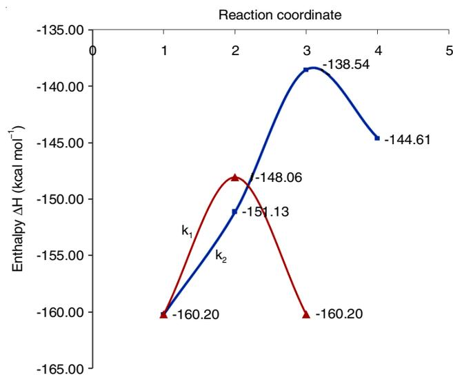
Fig. 2. Graph of enthalpy vs. reaction coordinate
