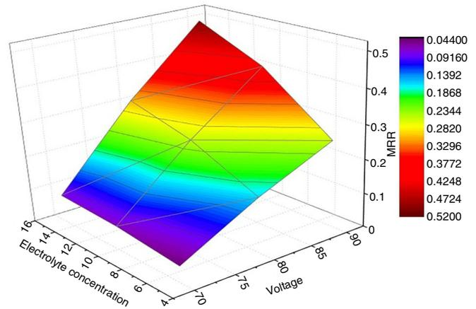
Fig. 3. 3D surface plot for material removal rate vs. voltage and electrolyte concentration
