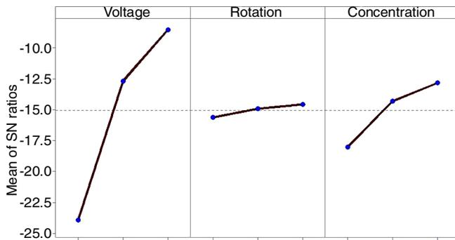
Fig. 2. Mean S/N ratios plot for material removal rate
