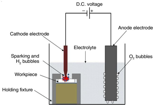
Fig. 1. Basic mechanism of electrochemical discharge machining
