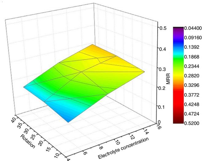
Fig. 5. 3D surface plot for material removal rate vs. electrolyte concentration and rotation
