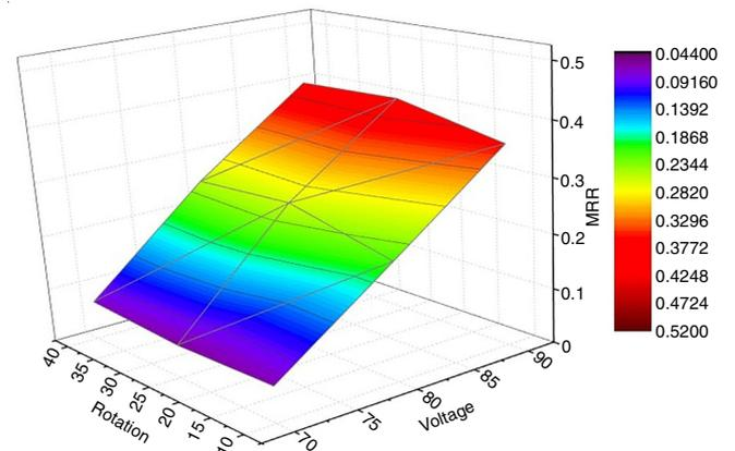
Fig. 4. 3D surface plot for material removal rate vs. voltage and rotation
