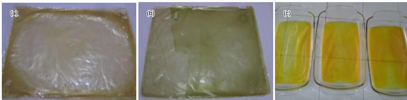
Fig. 1. Poly(lactic acid) based films modified with mangosteen skin (a), soursop leaves (b) and turmeric extract (c)
