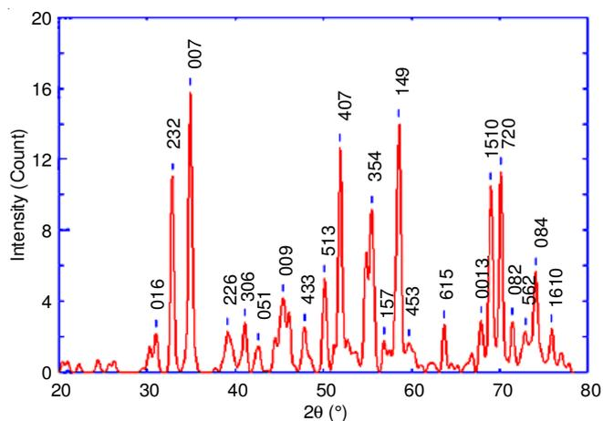
Fig. 2. Powder X-ray diffractogram of *bis*-thiourea nickel barium chloride crystal
