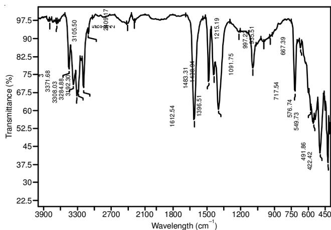
Fig. 4. FTIR spectrum of *bis*-thiourea nickel barium chloride crystal
