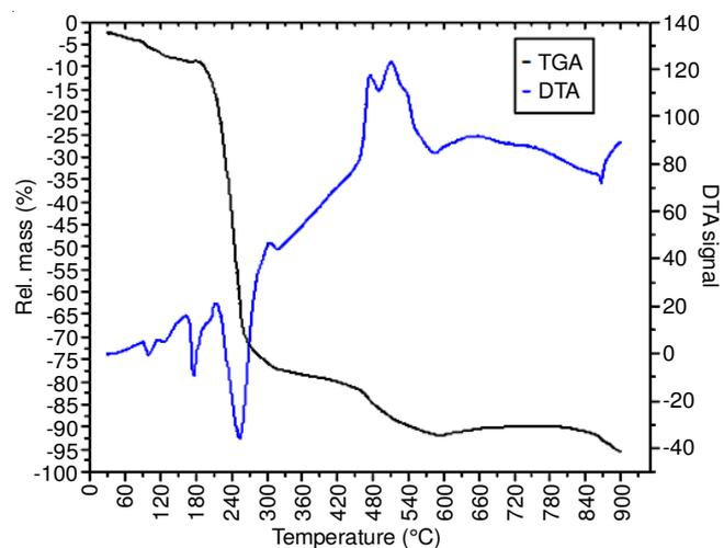
Fig. 5. TGA/DTA curve of BTNBC crystal
