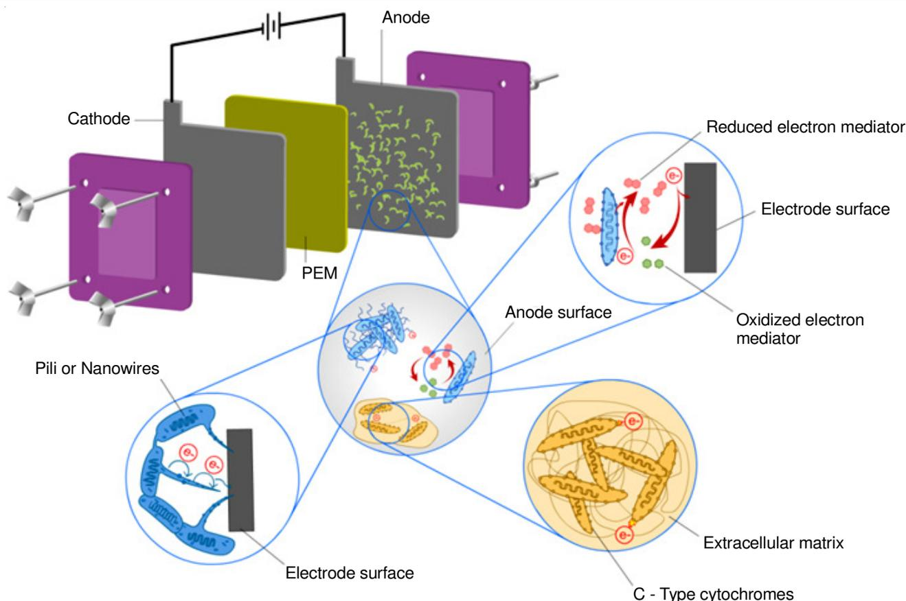
Fig. 3. A typical microbial fuel cell. Bacterial biofilm is formed on the anode surface that transfers electrons through any of the three modes: redox molecules, extracellular matrix, or pili. Cathode and anode are separated by proton exchange membrane
