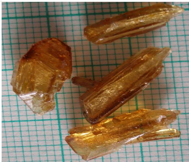
Fig. 1. Photograph of 3-nitroanilinium trichloroacetate crystal
