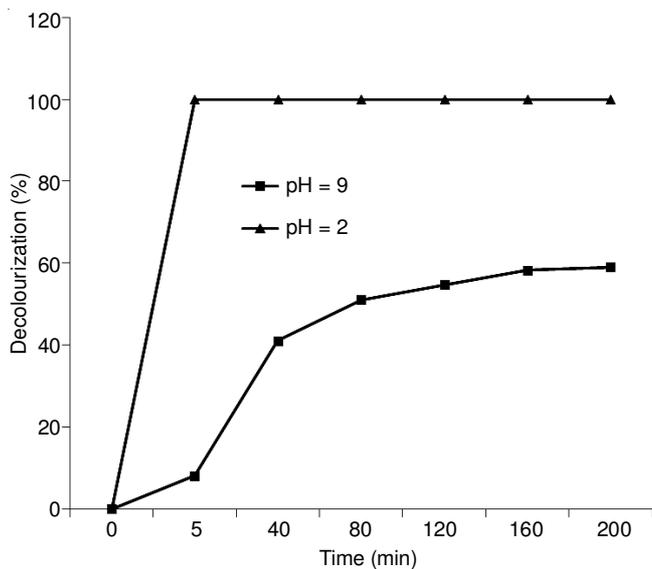
Fig. 4. Effect of pH on Eosin yellowish dye
