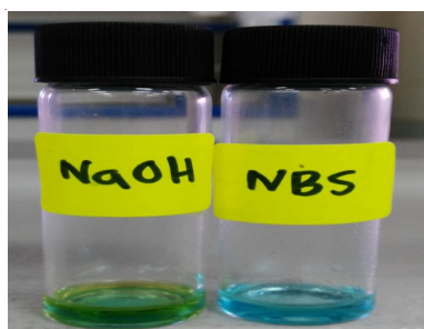
Fig. 2. Solution of FHA-metal complex using NBS and NaOH catalysts after left overnight. Reaction condition: reaction time 45 min, temperature 70 °C, agitation 150 rpm
