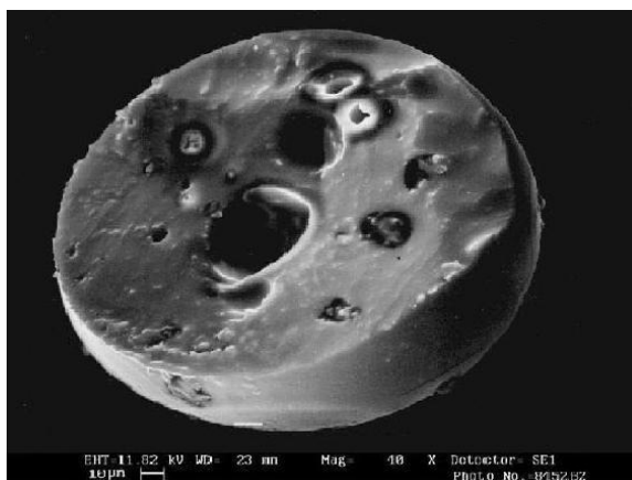
Fig. 3. Cross-sectional view of microsphere after dissolution
