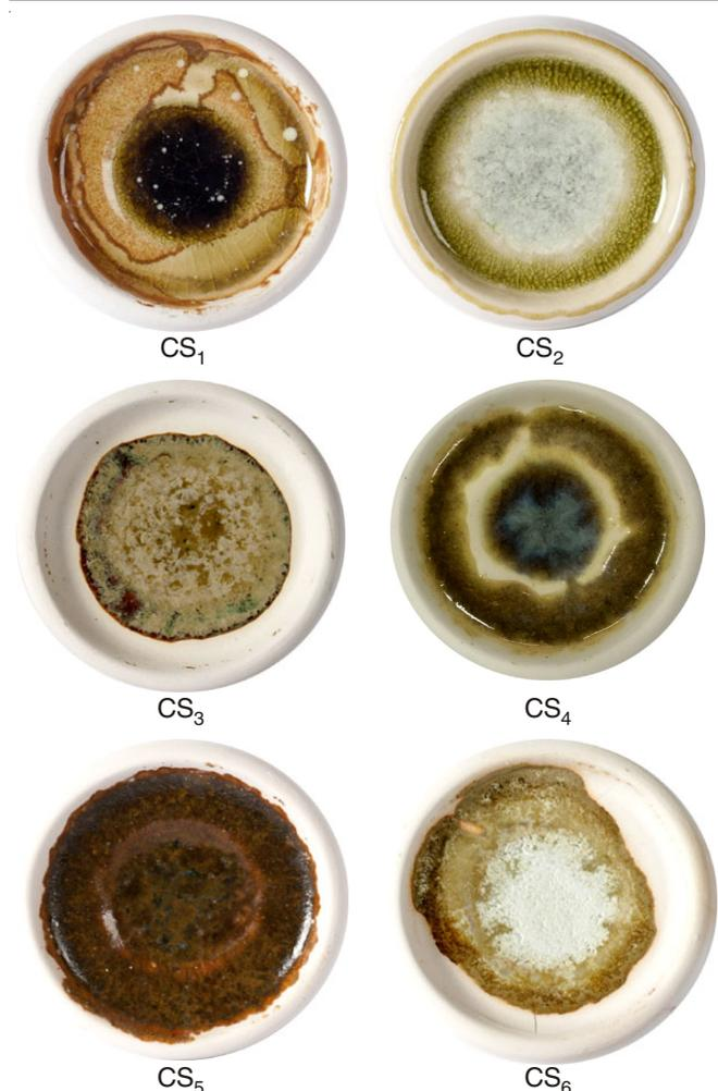
Fig. 3. Surface appearance and colour of the glazes prepared by copper slag fired at 1200 °C; CS<sub>1</sub>, CS<sub>2</sub>, CS<sub>3</sub>, CS<sub>4</sub>, CS<sub>5</sub> and CS<sub>6</sub>
